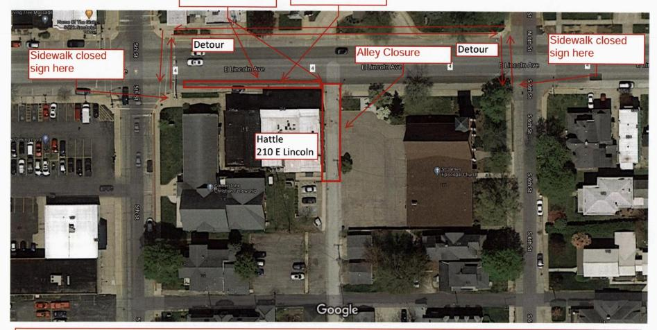
Lacasa is requesting sidewalk and alley closure around our property at 210 E Lincoln (The Hattle) starting Monday March 29th for 4 or 5 days. This is required for a brick mason, using a lift, to repair and replace brick prior to repainting the building.
